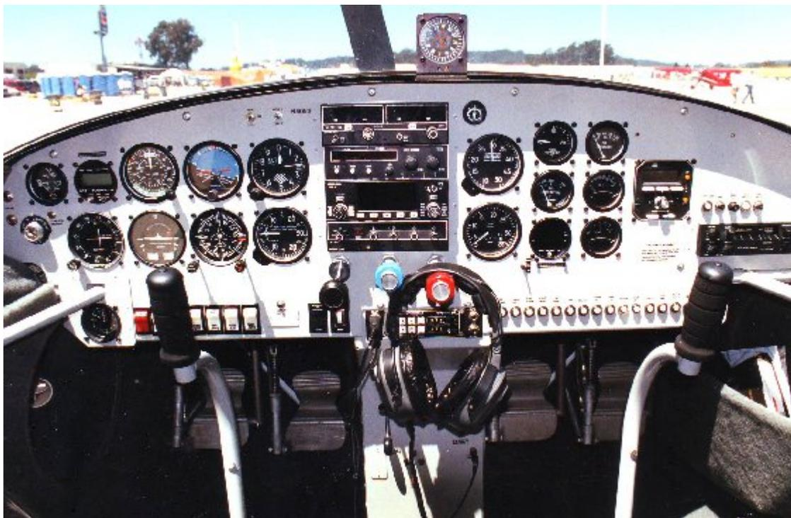
**The Stallion is equipped for flight into instrument conditions. A King KLN 90 is the centerpiece.**
